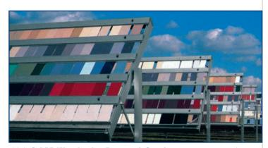
Sayerlack chose Florida because the climatic conditions in which **Q-LAB Weathering Research Service** operates are the most challenging for the tests to be carried out on the wood samples treated with outdoor paints
